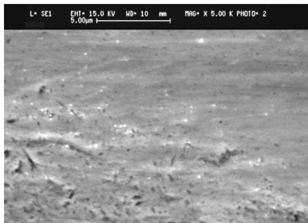
Fig. 6 SEM micrograph of a stainless steel sample after oxidation of two consecutive SAM layers
